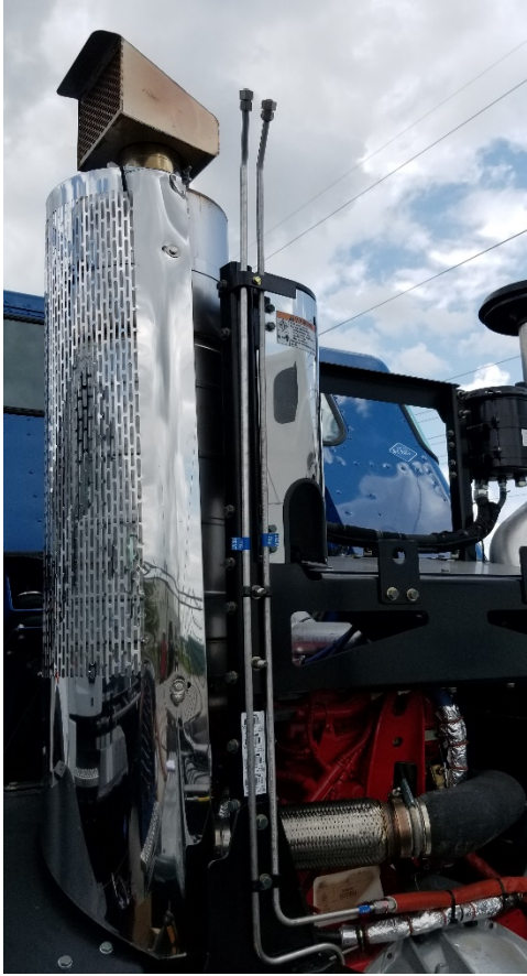
Figure 41: PRD Vent Installation
