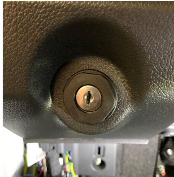
Figure 23: Key Switch Installed
