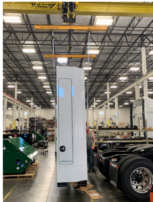
Figure 2: Correct Hoist Set Up
