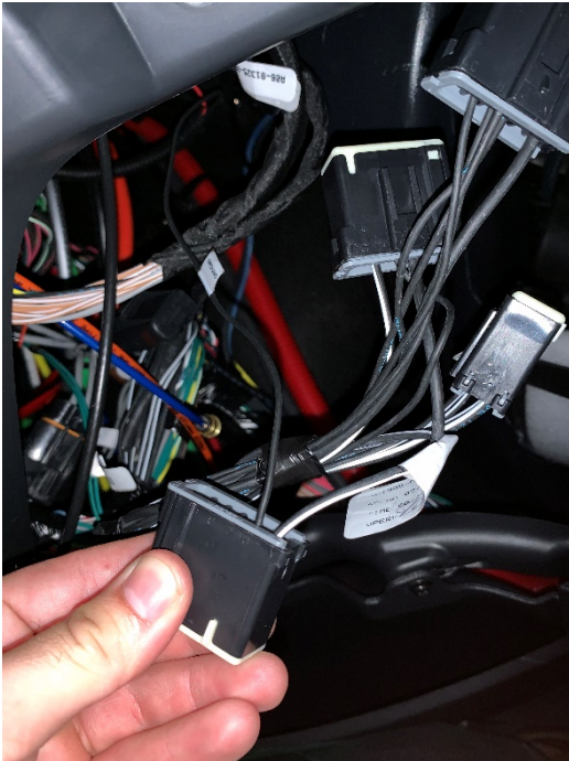
Figure 30: Ground Splice Blocks
