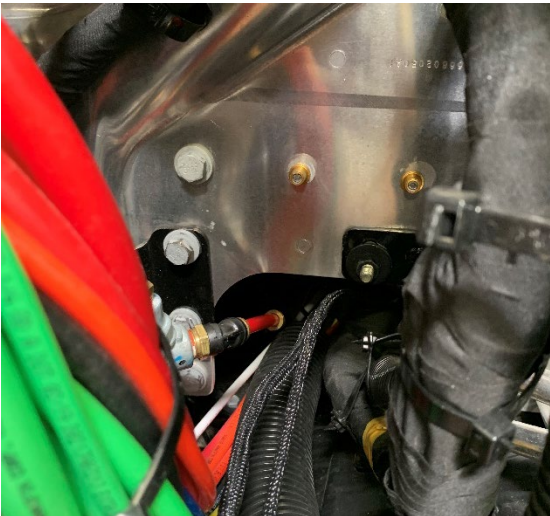
Figure 17: Wiring Harness Routing- Under Hood
