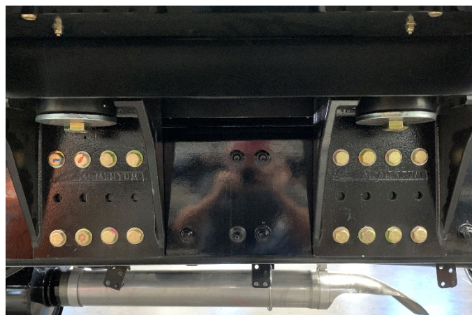
Figure 31: Final Torqued All Bolts
