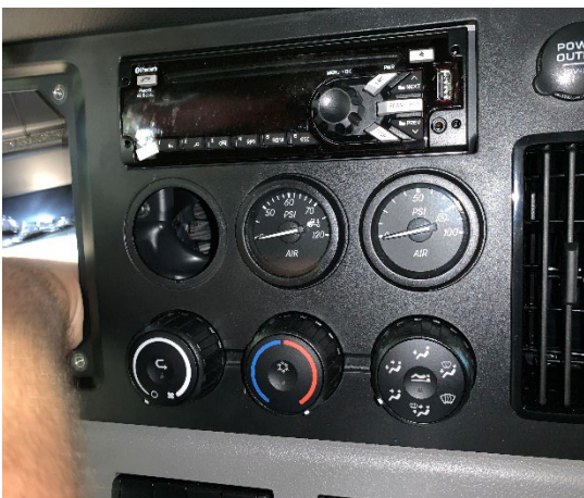
Figure 27: Fuel Gauge Blank Removed
