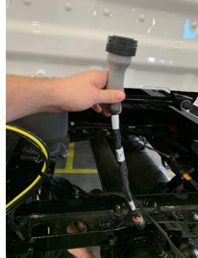
Figure 23: BOC Harness Install
