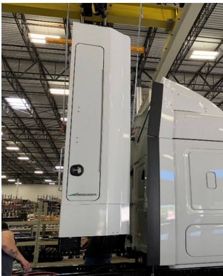
Figure 14: BOC Final Installation
