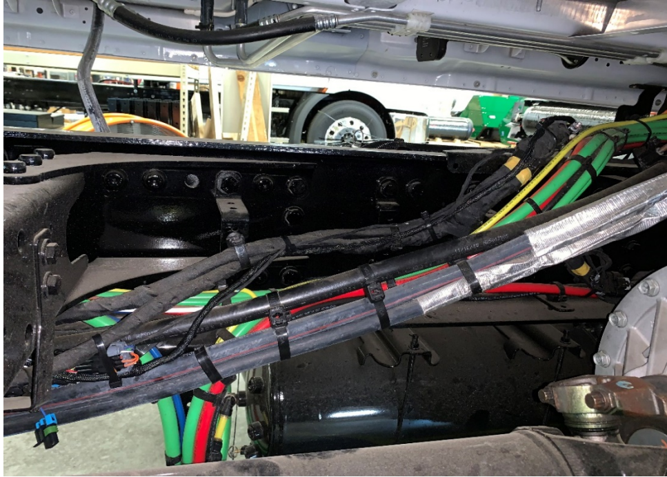
Figure 5: Wiring Harness Routing-Under Cab
