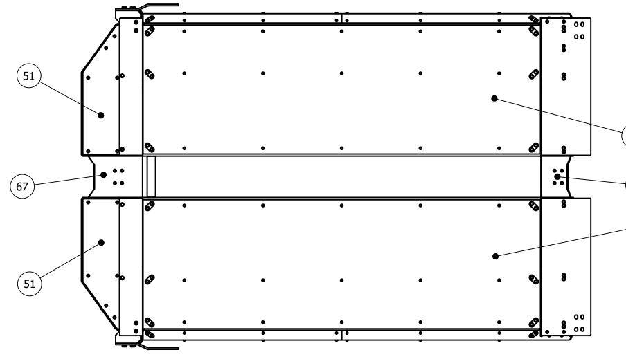
ALL DIMENSION TOLERANCES UNLESS NOTED ONE PLACE ±.06 .Χ TWO PLACES .XX ±.03 ±.010 THREE PLACES .XXX FOUR PLACES .XXXX ±.0010 ALL MACHINED SURFACES TO BE 250 RMS UNLESS NOTED.
