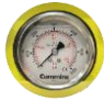
YELLOW labeled gauge is Supply pressure gauge indicates cylinder pressure if the cylinder valve(s) are open.
