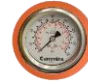
ORANGE labeled gauge is Regulated pressure gauge indicates the fuel pressure sent to the engine. With key on, the pressure should read approximately 80 psi.
